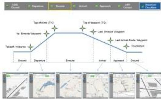
The EFB-system automatically switches from one chart to the logically next chart thus the **chart-type matches the current flight phase**.
